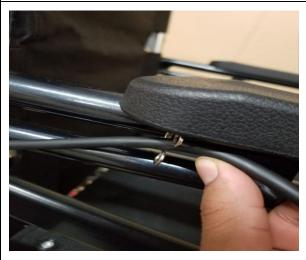
Before folding the chair make sure to release the back handleBar
